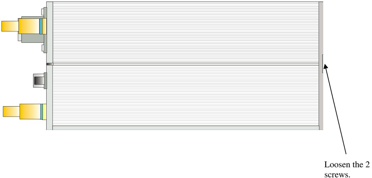
Lift the top part 30-45 degree from the bottom part and pull the top part in the direction of the arrow to release the hinge.
